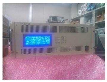
OCTAD (High speed sampler and DBBC)
